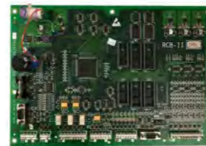
OTIS RCB-II board GHA21270A1
